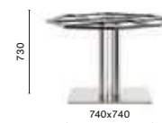
COLUMN 4x Ø 76 TOP MAX 1600x1600; Ø 2000
